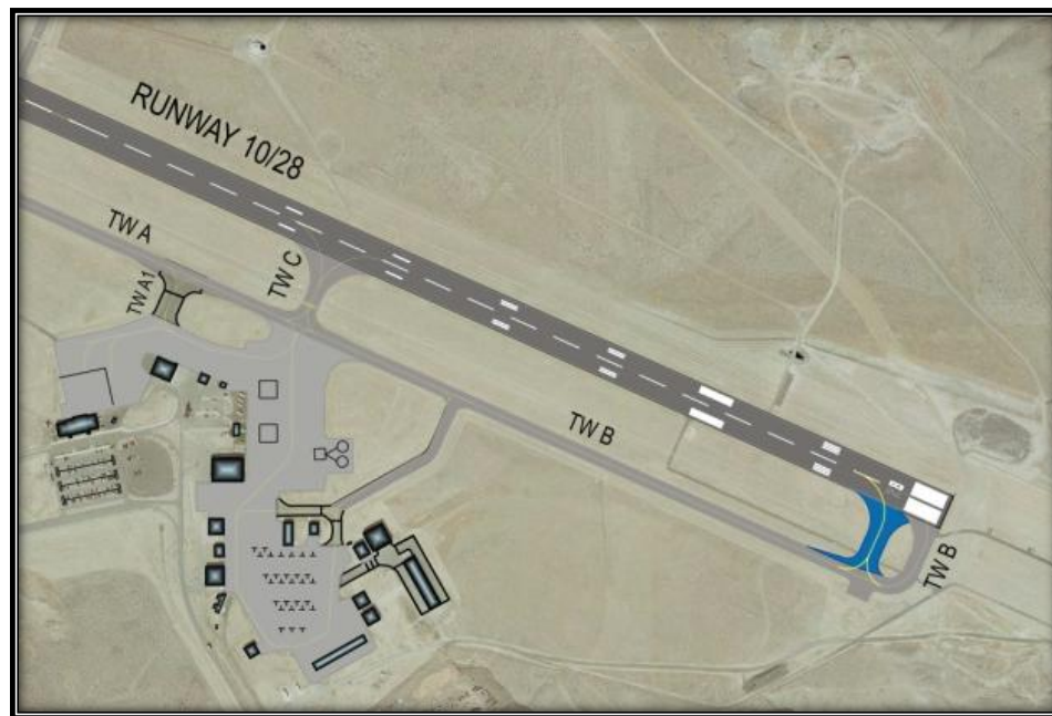
FIGURE 7-1 - BYPASS AND CONNECTOR TAXIWAY
